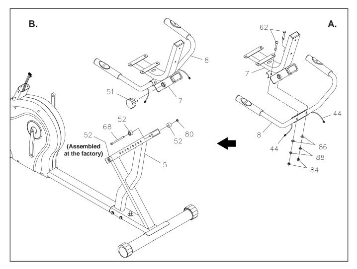
NOTE: Be careful not to damage the PULSE SENSOR WIRES(44) when attaching the HANDRAIL(8) and the SEAT FRAME(7).
